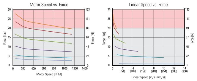
Note: All motor load curves were generated with a 40 VDC, 2-phase ON driver and full stepped at the motor rated current. They account only for motor performance - different nut and motor combinations may yield different performance characteristics. Performance plots for other lead screw and motor winding configurations can be generated at www.thomsonlinear.com/smla.
