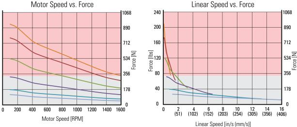
Note: All motor load curves were generated with a 40 VDC, 2-phase ON driver and full stepped at the motor rated current. They account only for motor performance - different nut and motor combinations may yield different performance characteristics. Performance plots for other lead screw and motor winding configurations can be generated at www.thomsonlinear.com/smla.
