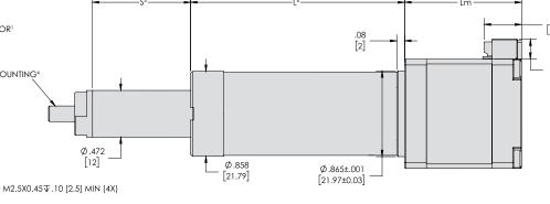
1. Molex 53253-0670 connector shown. Wire harness with Molex 51065-06000 mating connector and flying leads included with motor. For wiring diagram and connector details, see page 46.
