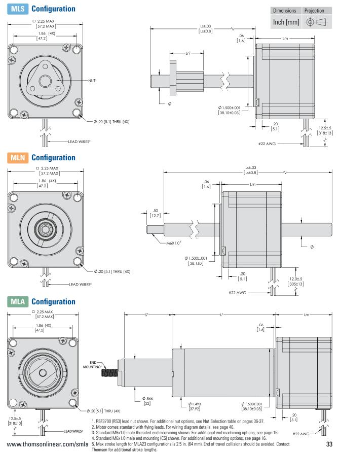
6. Cover tube length (L) = stroke (S) + 1.74 in. (44.2 mm).
