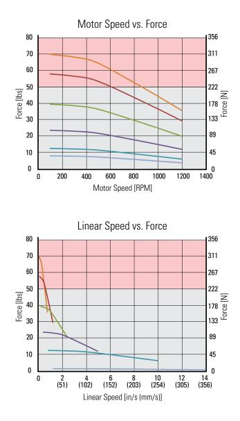
Note: All motor load curves were generated with a 40 VDC, 2-phase ON driver and full stepped at the motor rated current. They account only for motor performance - different nut and motor combinations may yield different performance characteristics. Performance plots for other lead screw and motor winding configurations can be generated at www.thomsonlinear.com/smla.
