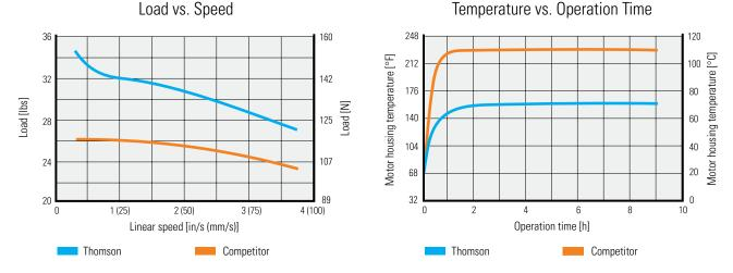
The curves where generated with a 1.5 A / 2.33 V, 1.8° NEMA 17 single stack, rotating screw stepper motor. Test ran with a 0.9°, 24 VDC chopper drive and a 4-2516 lead screw at an ambient temperature of 20 °C.
