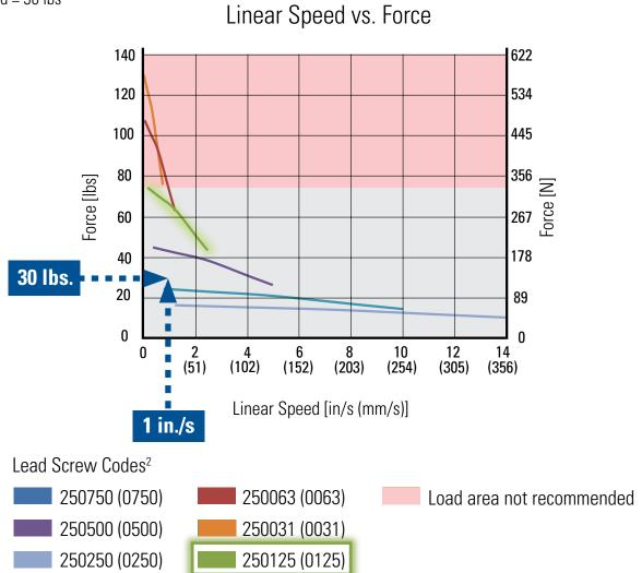
Given the speed and load requirements of 1 in./s and 30 lbs., respectively, a motor with a 0.25 in. diameter x 0.125 in. lead (250125) will be a sufficient stepper motor linear actuator assembly for this application<sup>3</sup>.
