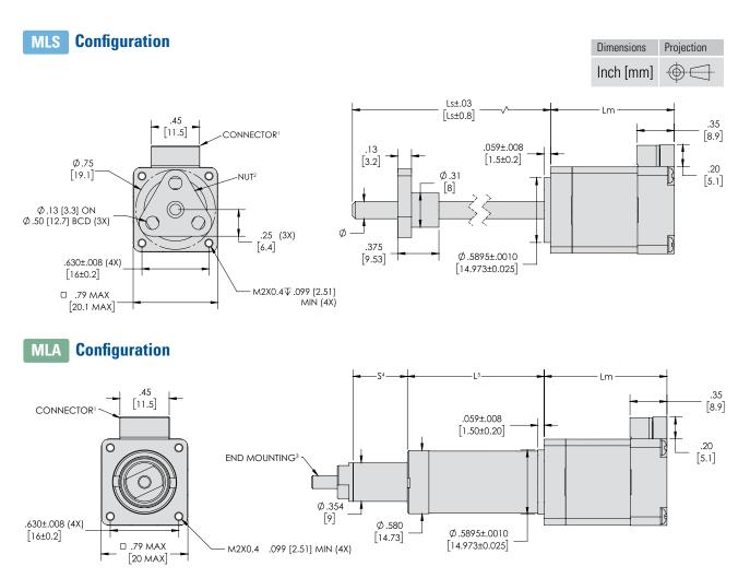
1. S6B-ZR(LF)(SN) connector shown. Wire harness with JST ZHR-6 mating connector and flying leads included with motor. For wiring diagram and connector details, see page 46.
