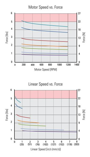
NOTE: Motor load curves were generated with a 24 VDC, 2-phase ON driver and half stepped at the motor rated current. They account only for motor performance - different nut and motor combinations may yield different performance characteristics. Performance plots for other lead screw and motor winding configurations can be generated at www.thomsonlinear.com/smla.
